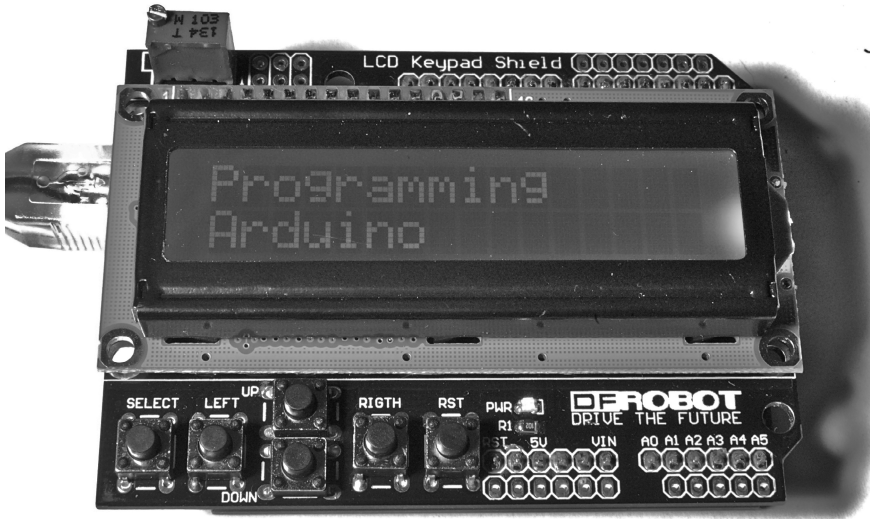
Figure 9-2 LCD shield attached to an Arduino board.
