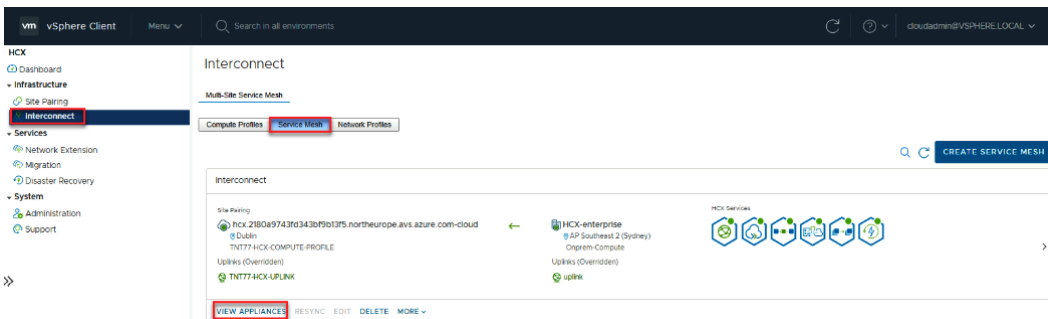
Figure 5.36 – Viewing Service Mesh appliances status
