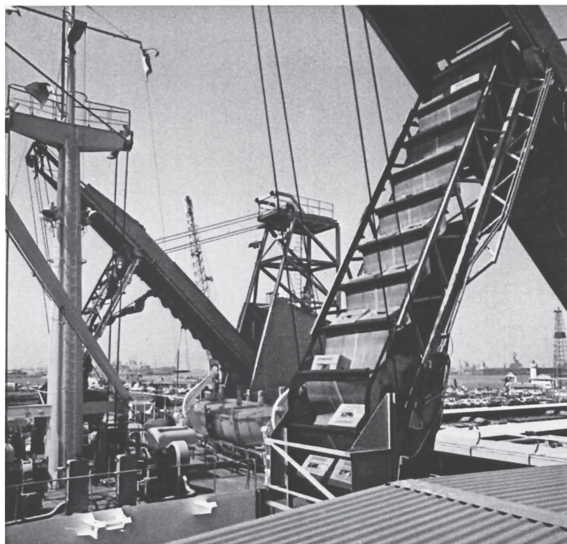
FIGURE 22. Boxed bananas being unloaded from a ship by conveyor belt in the Port of Long Beach, 1967. Courtesy Port of Long Beach.
