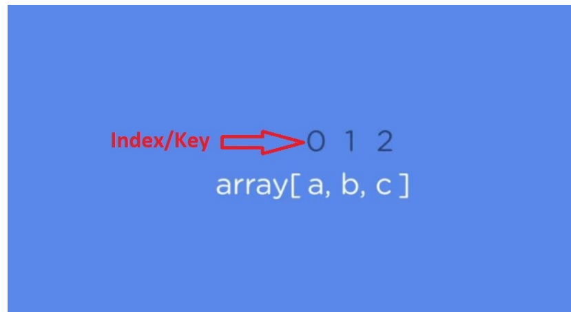
Figure 2.2.1: An example of an array with its values (a, b, c) and keys (0, 1, 2)
