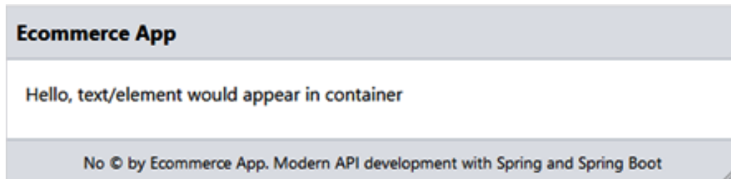
Figure 7.2 – Basic structure of app containing Header, Footer, and Container components
