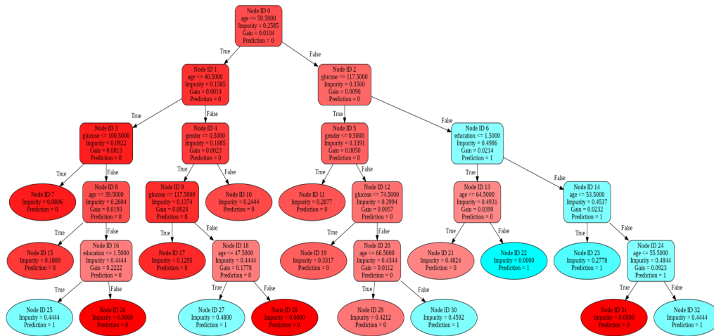
Figure 5.73: The tree diagram of the trained DTC model
