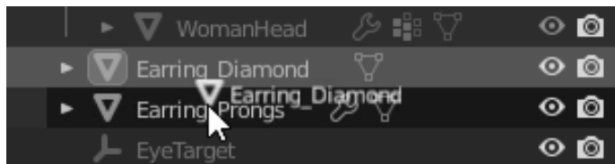
Figure 8.14 – The Earring_Diamond object being dragged on top of the Earring_Prongs object in the Outliner (hold Shift before releasing)
