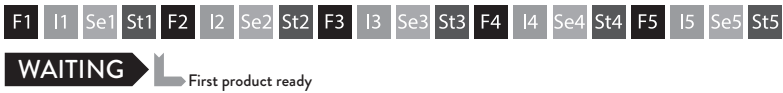
Figure 7: Simulation of “envelope game” (fold, insert, seal, and stamp the envelope) (Source: Stefan Luyten, “Single Piece Flow: Why mass production isn’t the most efficient way of doing ‘stuff’,” Medium.com, August 8, 2014, https://medium.com/@stefanluyten/single-piece-flow-5d2c2bec845b#907sn74ns .)
